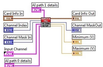
**M4i Cluster Input Channel Settings / (element ai channel.ctl)**
