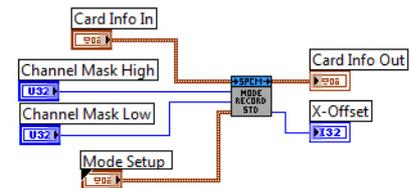
**Cluster Record Mode Standard Setup / (element mode.ctl)**
