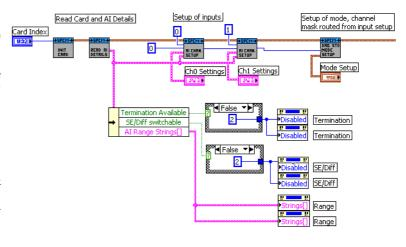
Finally the "DAQ std mode setup" set's the current mode and also programs the channel mask that has been modified by the two channel setup VIs.
