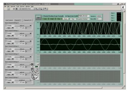
The card setup is splitted into three pages to group them for easier use. On the "Card Control" page all settings are placed that are related to the card like clock, memory or mode setup. The other two pages contain the complete analog setup for 8 channels each.
