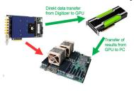
For applications requiring high performance signal and data processing Spectrum offers SCAPP (Spectrum's CUDA Access for Parallel Processing). The SCAPP SDK allows a direct link between Spectrum digitizers, AWGs or Digital Data Acquisition
