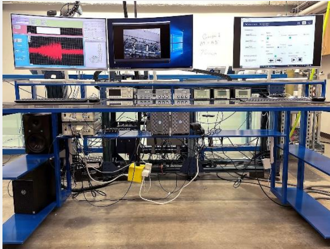
Figure 3: The control console with the two grey PCIe chassis in the middle
