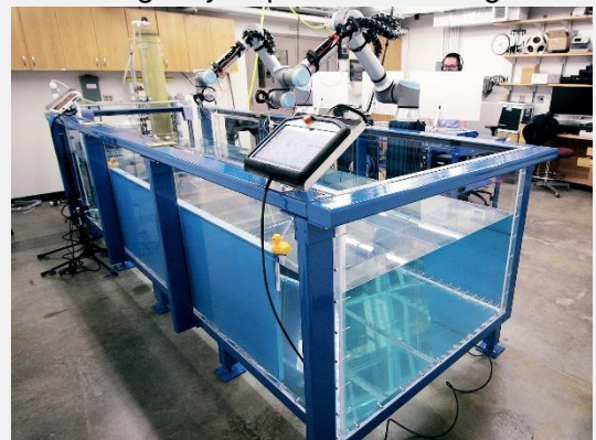
Figure 1: The water tank with the two robotic arms to position the transmitter and receiver
