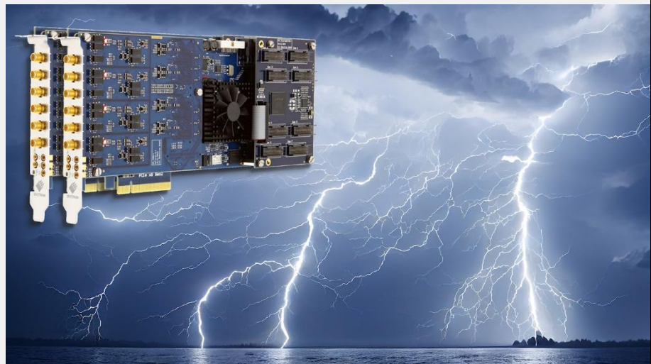
Figure 1: Two M4i.4451-x8 digitizers synchronized for lightning research
