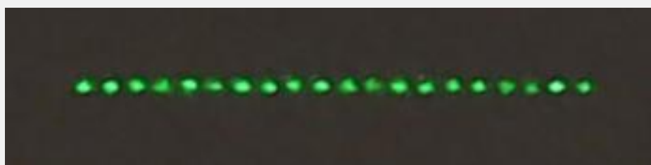
Figure 5. Camera image of a screen with the 1 st -order diffraction pattern of a laser. The laser is passing through an AOD that is supplied with a multi-tone signal with 20 carriers.
