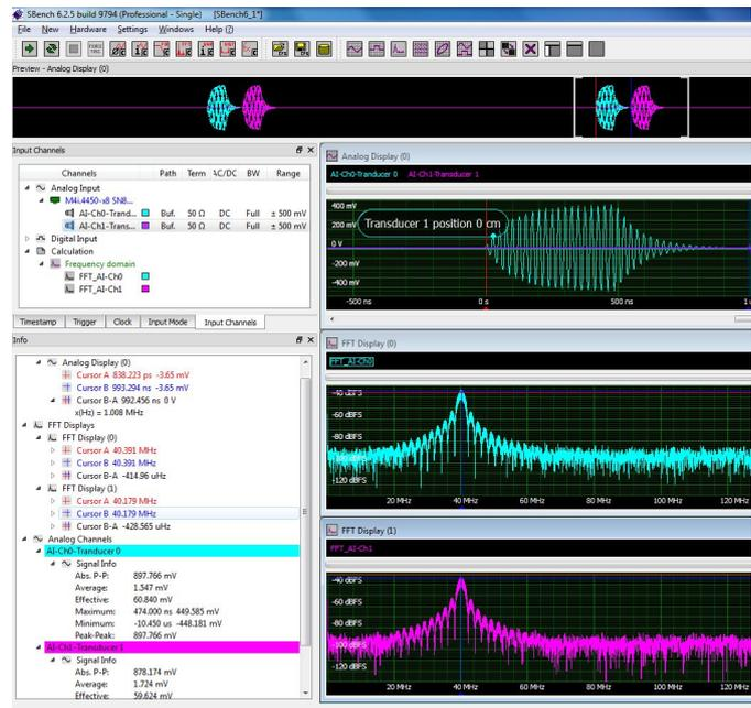
SBench 6 is a powerful and intuitive interactive measurement software. Besides the possibility to commence the measuring task immediately, without programming, SBench 6 combines the setup of hardware, data display, oscilloscope, transient recorder, analysing functions and export functions under one easy-to-use interface. All current Spectrum digitizerNETBOX and generatorNETBOX products, all M2p, M2i, M3i, M4i, M4x and M5i cards as well as all MI, MC and MX data acquisition cards are supported.
