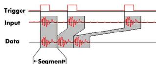
The Multiple Recording mode allows the recording of several trigger events without re-starting the hardware. With this option very fast repetition rates can be achieved. The
